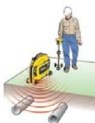
Induce a signal to locate utilities.
