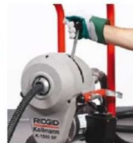
Release handle, cable stops instantly
