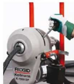
Engage clutch, cable spins
